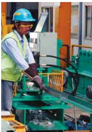
Truss components are manufactured
