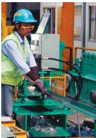
Truss components are manufactured
